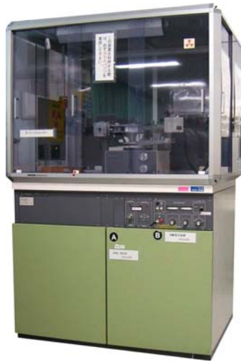
XRD (X-ray diffraction, X線回折) 装置と装置模式図
