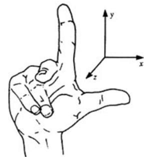
FIGURE 1.28 The right-handed rule for labelling axes.
